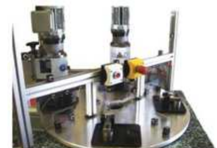
Rotary riveting station to secure the terminals on a capacitor using two radial riveting machines RN 081
