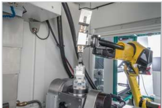
PICOMAX 75 with modular 6-axis articulated arm robot for blank parts handling
