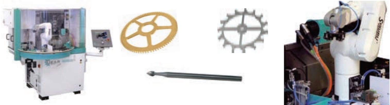
Gear hobbing center with robot automation and various feed systems such as palletizing system, feeder bowl, conveyor belt and image recognition etc.
