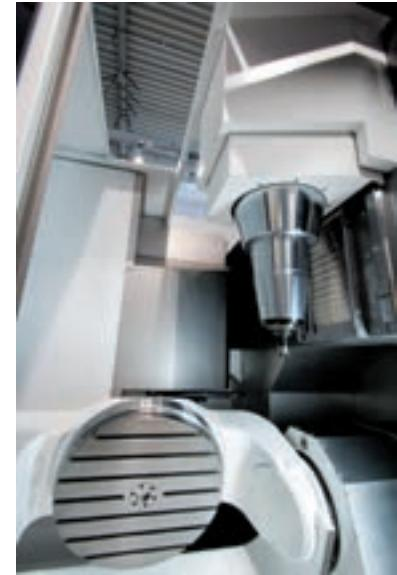
HSC gantry machining centre of 5 axes design
