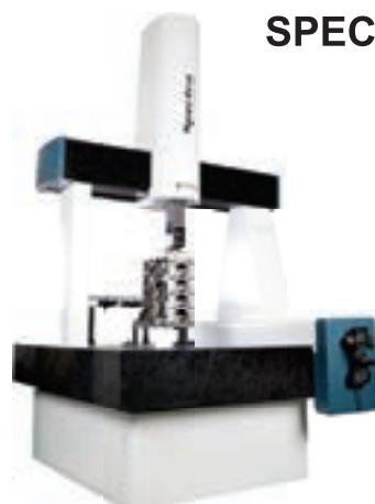
Large measuring range bridge type CMM. Using special techniques for machining and grinding of granite guides, we are able to achieve accelerations similar to lighter construction machines with further benefit of naturally stabilised material.
