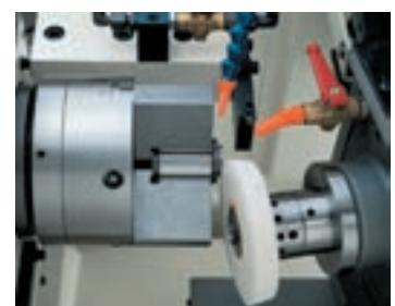
Die VOUMARD VM 110 is a universally deployable internal and external circular grinding machine which is equally suited for one-off machining or series production of workpieces with small and intermediate dimensions
