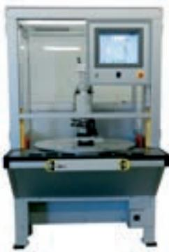
CNC coordinate riveting machine with round indexing table as a complete and autonomous workstation
